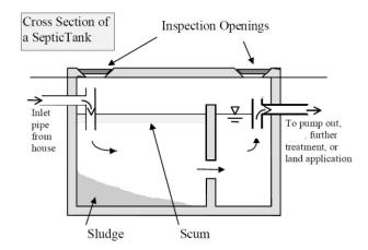
Bacteria in the septic tank break down the solid matter in the sludge and scum layers. Material that cannot be fully broken down gradually builds up in the tank and must be periodically pumped out.
