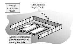
Such application systems have the potential to contaminate groundwater and are not recommended in sensitive locations or in higher density developments. Further treatment followed by subsurface irrigation should be considered.
