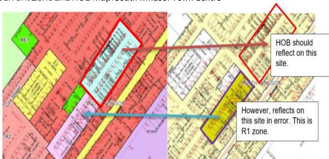
Figure 22 – Subject Site indicating anomaly
