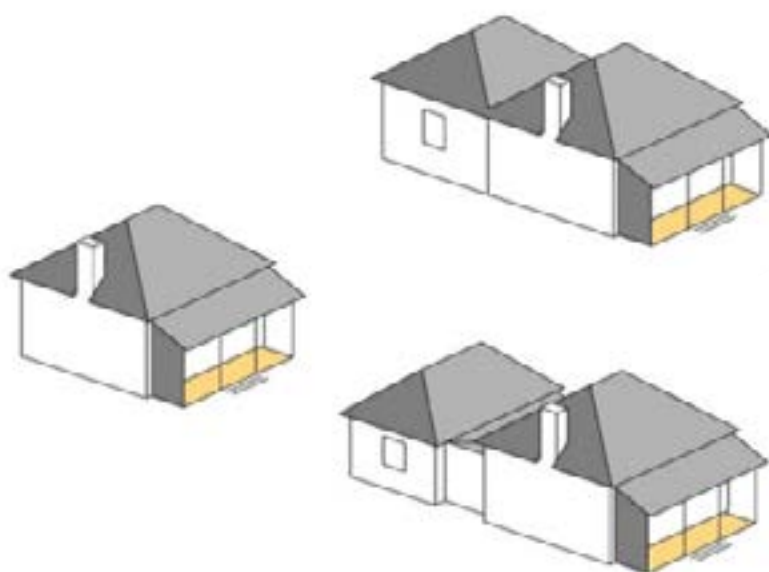
Suitable ways of extending an original building by not disturbing the original roof form and profile
