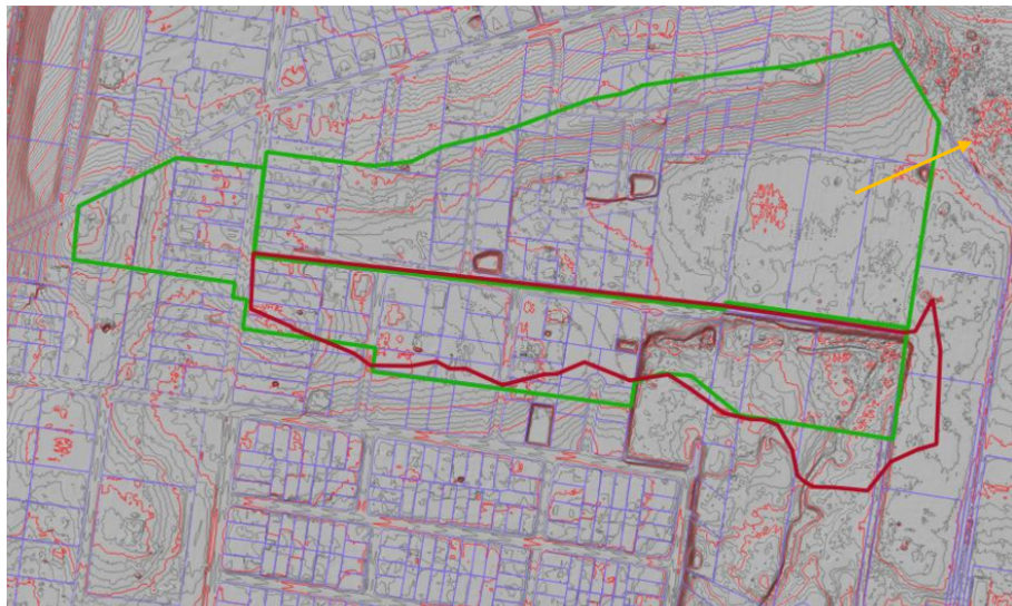
Figure 1 – Catchment area modelled by Cardno in green, actual catchment as of 2018 in red
