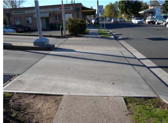
Figure 8.13: Driveway pavement with vehicle priority at interface with pedestrian path
