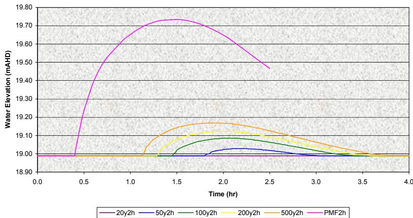
Figure 18 : Water Elevation Hydrograph at Point H10
