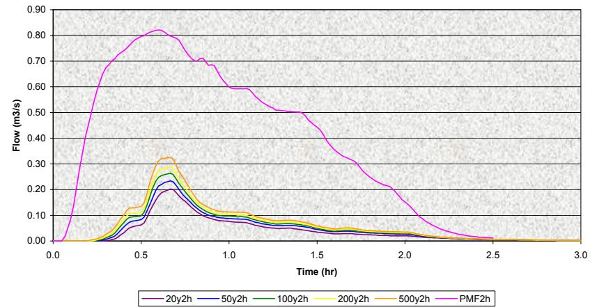
Figure 25a : Flow Hydrograph at Point H18
