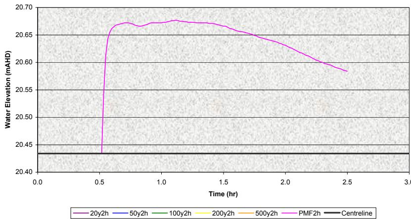
Figure 22 : Water Elevation Hydrograph at Point H15
