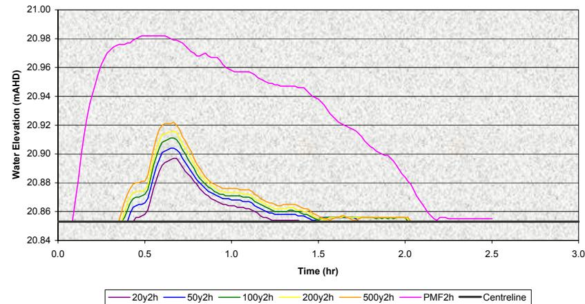
Figure 25 : Water Elevation Hydrograph at Point H18
