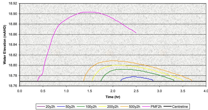
Figure 17 : Water Elevation Hydrograph at Point H9
