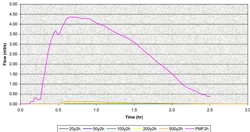
Figure 12a : Flow Hydrograph at Point H2
