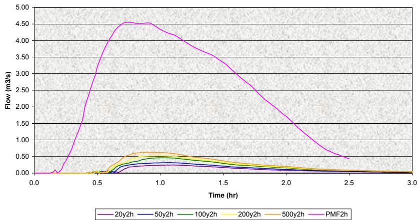
Figure 14a : Flow Hydrograph at Point H4
