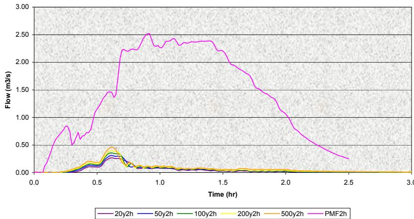
Figure 24a : Flow Hydrograph at Point H17
