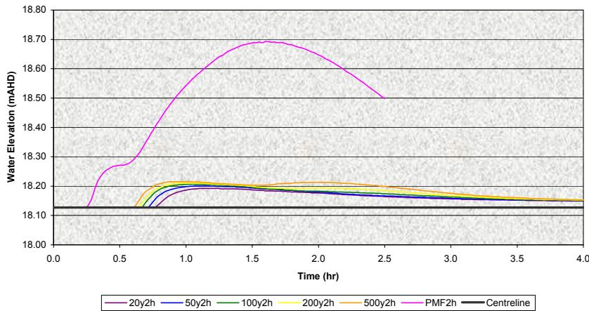
Figure 16 : Water Elevation Hydrograph at Point H8
