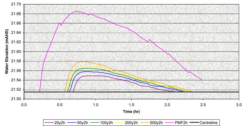
Figure 11a : Flow Hydrograph at Point H1
