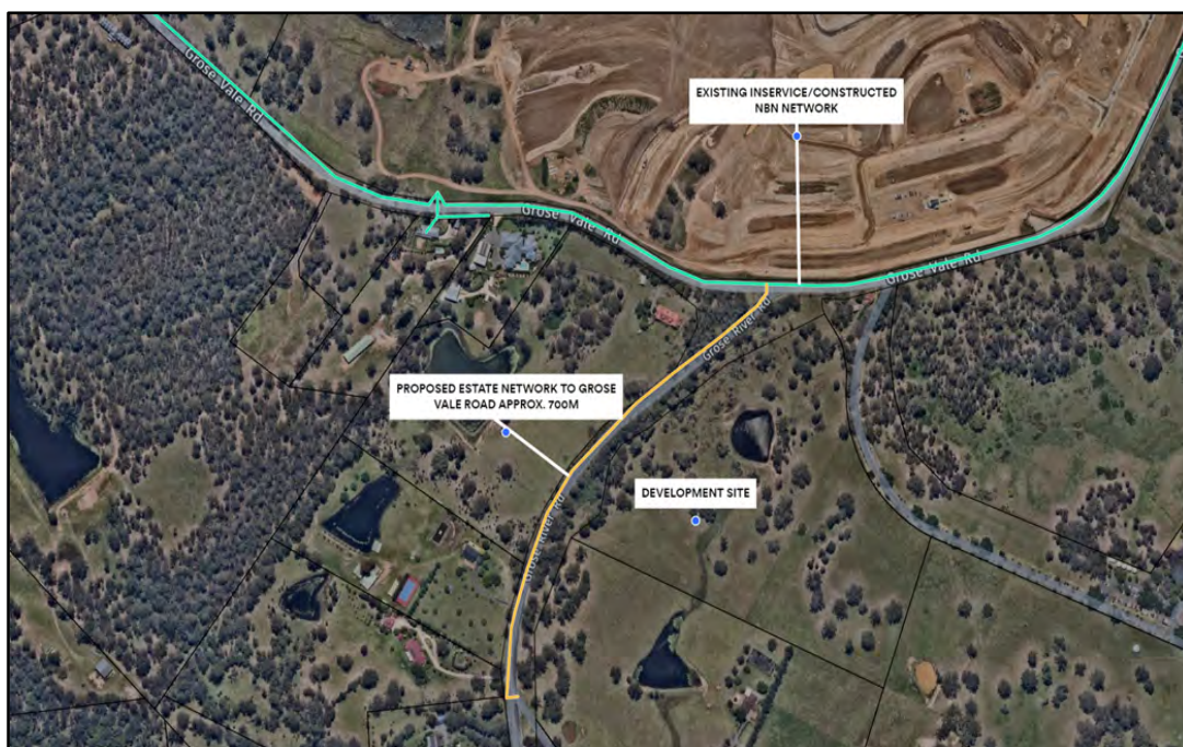
Figure 12: Indicative NBN lead in route
