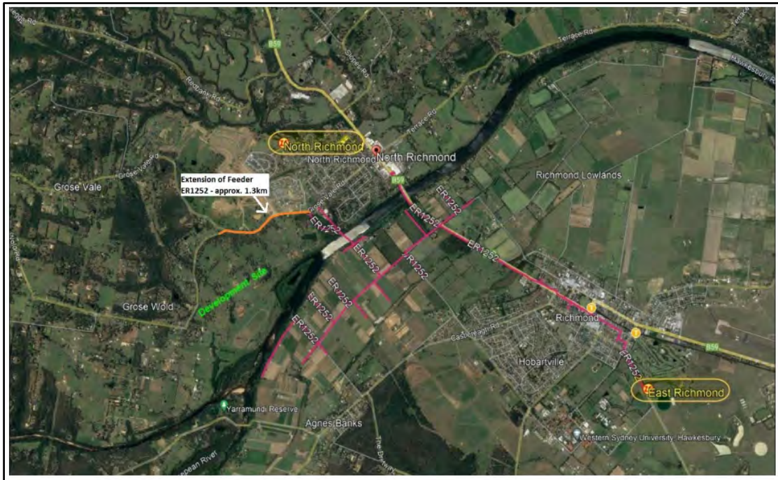
Figure 9: Indicative Feeder Route East Richmond Zone Substation
