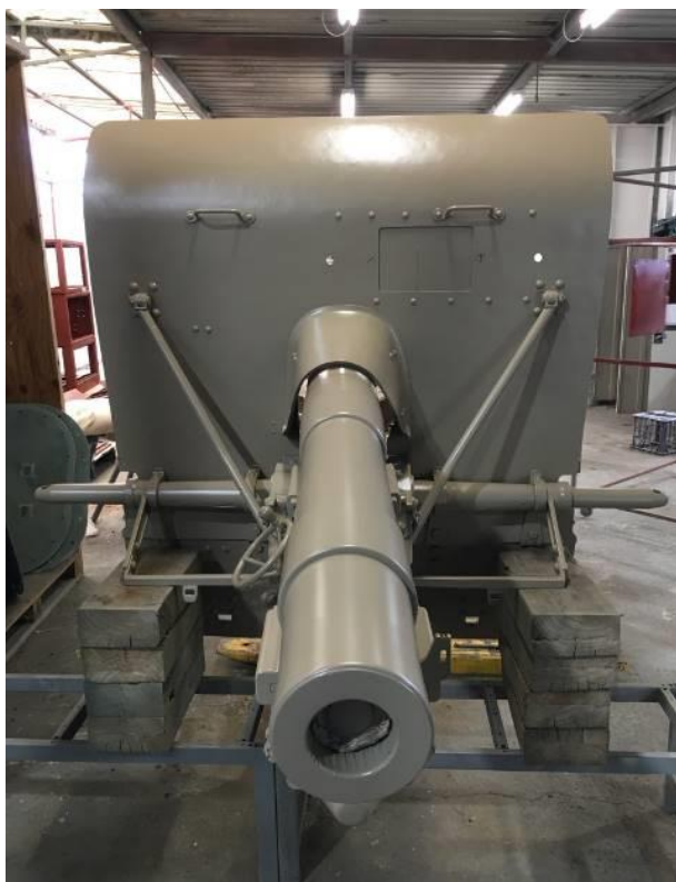
Figure 23 Final coating to shield and nozzle
