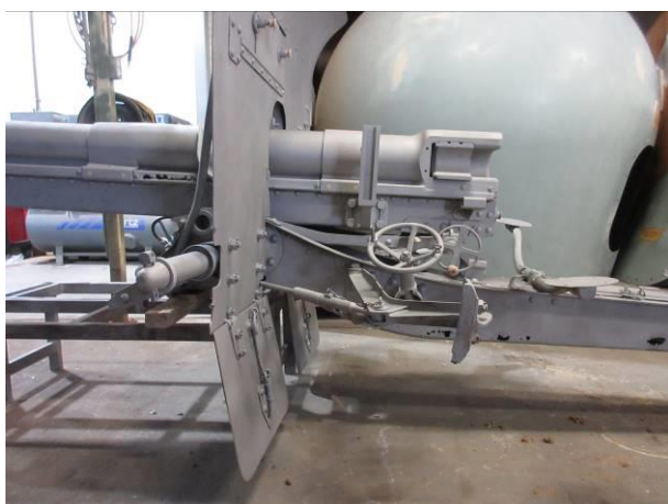
Figure 17 Gun section primed
