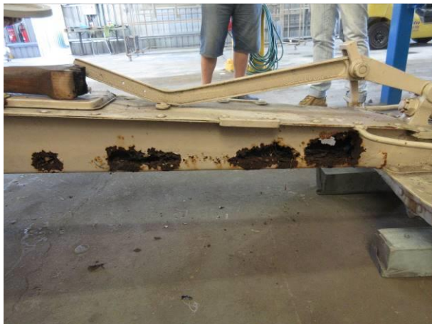
Figure 3 Corrosion on trail
