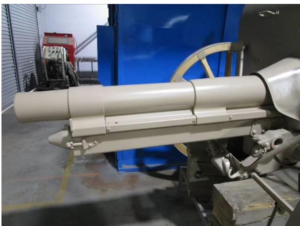
Figure 11 Gun barrel with new sleeves installed
