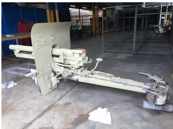
Figure 5 Intermediate coating and new trail skin
