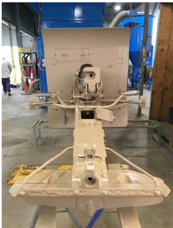
Figure 24 Final coating to trail and rear
