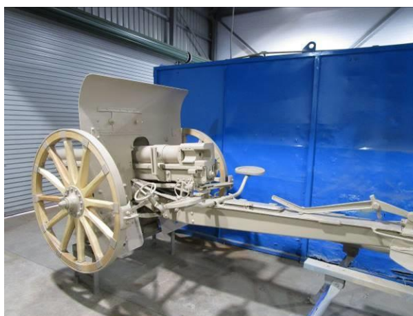
Figure 18 Completed final coating of gun
