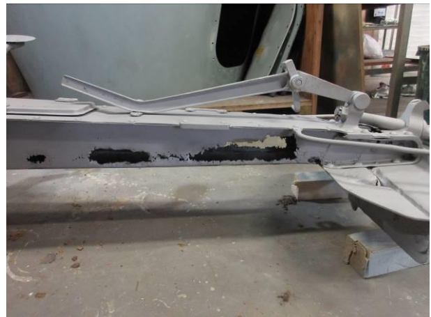
Figure 4 Abrasive blasting of trail
