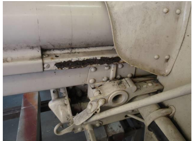
Figure 8 Corrosion on nozzle sleeves
