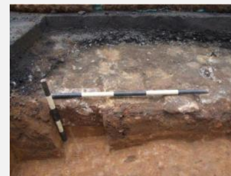
West-facing section view in Test Pit SA18 of the Telford type road base layer overlying the bedding material, followed by natural clay (AAJV 2017, p.76 Figure 50)
