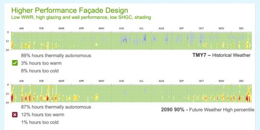
Figure 29: Modelled thermal autonomy for a high performance envelope apartment in Western Sydney, using both recent weather (TMY7 case) and predicted weather (2090 90% case) (Brannon 2018).
