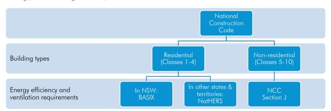
Figure 40: Energy efficiency and ventilation requirements for Australian buildings are defined by different codes depending on the building type and the state/territory
