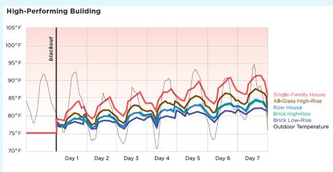
High-performing brick buildings, including the row house and brick low- and high-rise apartments, would stay below 80°F for the first half of the week, and never go above 85°F. The high-performing glass building reaches 88°F and the single-family house still rises above 90°F.
