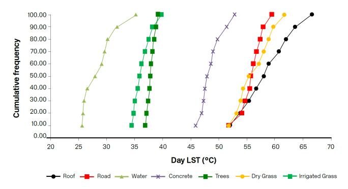
Figure 24: Temperatures of different urban surfaces (CRC for Water Sensitive Cities, 2020)
