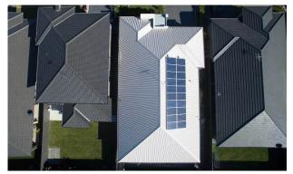
Figure 14: In general, lighter coloured roofs are cooler, with higher SRI
