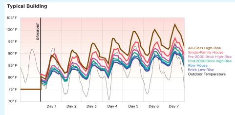
The typical all-glass high-rise apartment and single-family house heat to almost  $90^{\circ}F$  on the first day. The all-glass apartment climbs above  $95^{\circ}F$  on the fourth day and peaks over  $100^{\circ}F$ . The brick buildings, including the row house, low-rise and high-rise apartments, stay cooler throughout the week but still end above  $85^{\circ}F$ .
