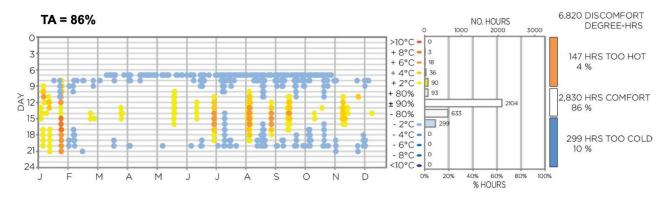
Figure 25: Thermal autonomy reporting example (Levitt et.al, 2013). In the dot plot portion of the diagram (left), blue dots represent hours Too Cold, while yellow and orange dots represent hours too hot. The Discomfort degree-hour total combines hours of discomfort with intensity of discomfort into a secondary but less precise metric of discomfort.
