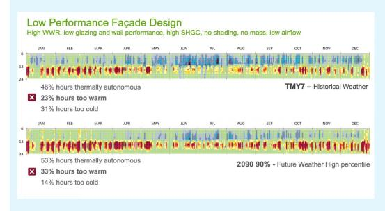
Figure 28: Modelled thermal autonomy for a minimally code-compliant apartment in Western Sydney, using both recent weather (TMY7 case) and predicted weather (2090 90% case) (Brannon 2018).
