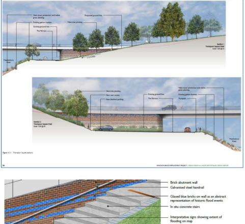
Blue resin inlays on concrete strip reflect the recorded flood levels Metal inlays on stairs interpret the level of water historic flood events
