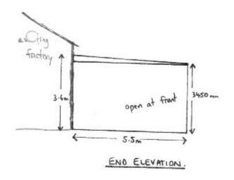
Material: Walls 80mm coolroom panel Roof: 100mm coolroom panel.
