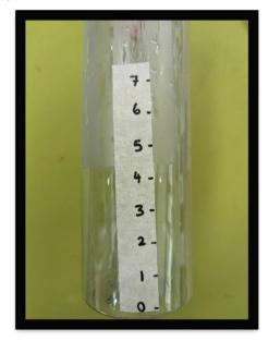
5. Because bottles aren't flat on the bottom, we need to pour a bit of water into our bottle to have a flat, even surface to begin measuring rainfall from. This will mean our measurements are more accurate!
