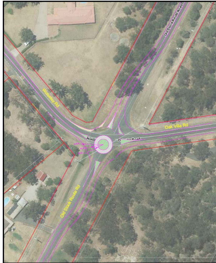
Figure 4: Proposed Design Concept - realignment of Old Stock Route Road with Roundabout
