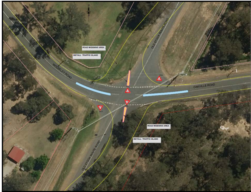
Figure 3: Proposed Design Concept – realignment of Old Stock Route Road with concrete median Islands
