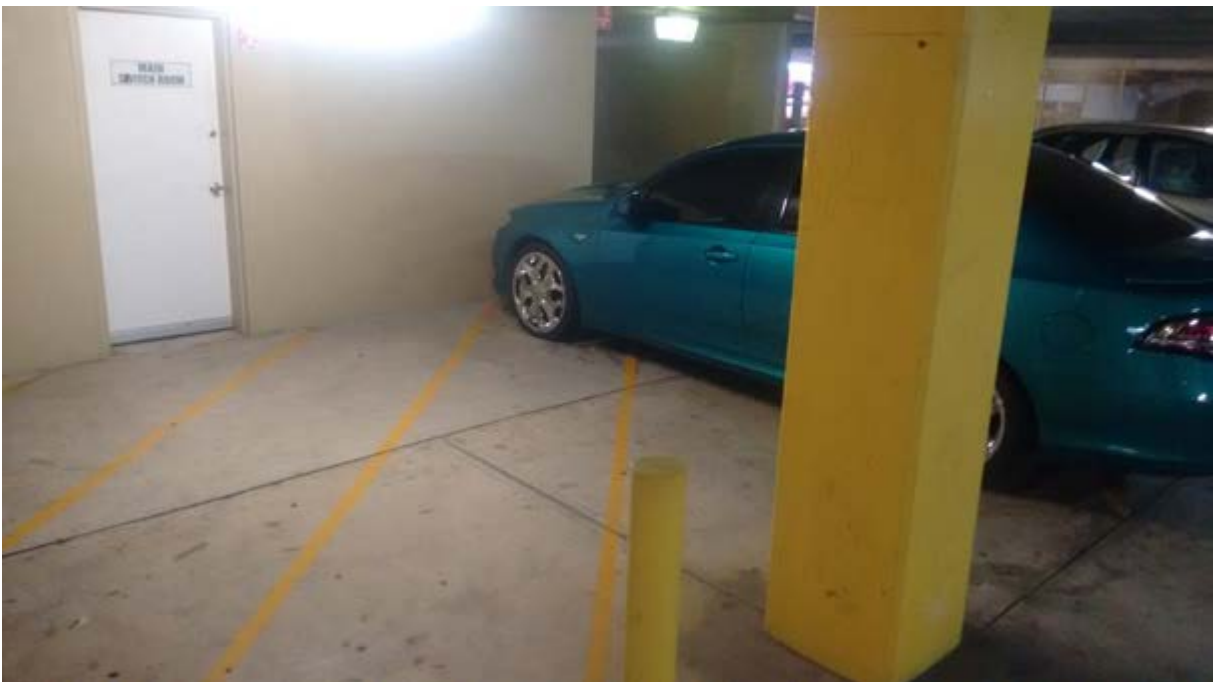
Figure 6: Hatched area suggesting no parking is permitted. No signs and no bollards exist to prevent the parking of vehicles in this area.
