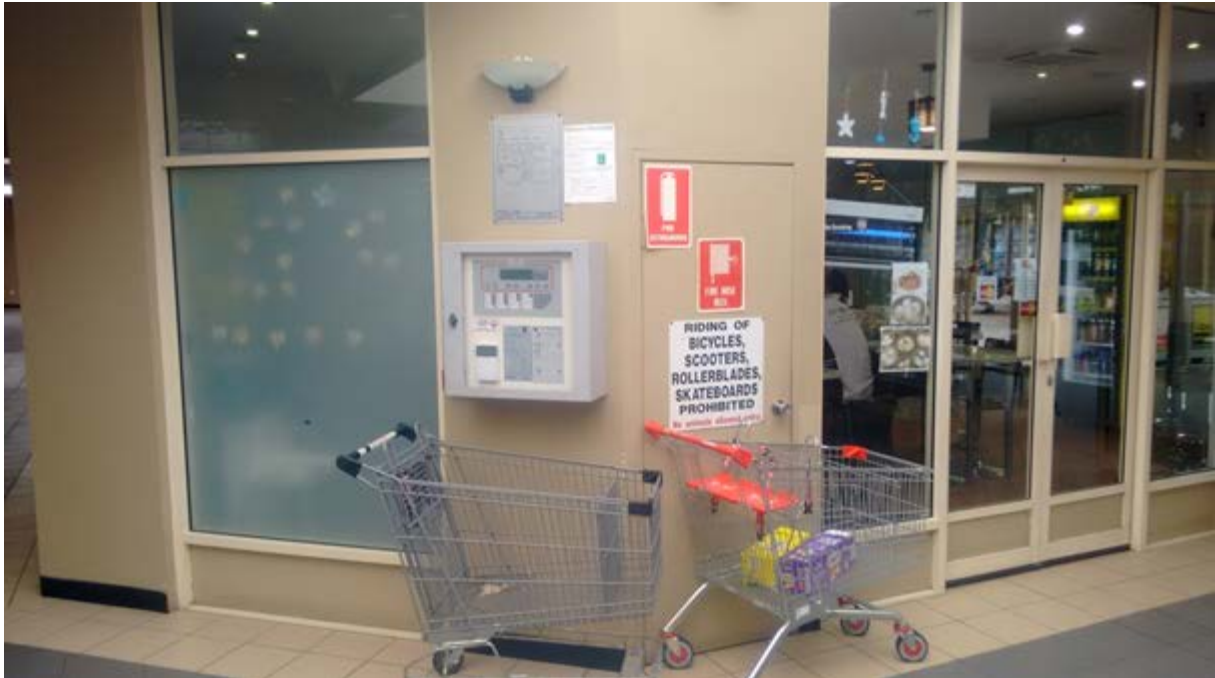
Figure 2: Outside shop 4 showing shopping trolleys obstructing access to Fire Hose Reel room.
