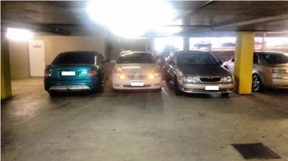
Figure 3: Vehicles parked in hatched area restricting pedestrian access to fire escape door behind.
