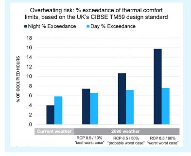
Figure 30: Current and future annual overheating risk to a bedroom with a high performance building envelope, without using air conditioning. The three 2090 cases reflect arrange of future weather models and show that thermal comfort and safety will be particularly vulnerable to night time temperature increase. Intermediate time forecasts were not modelled. (Brannon, 2018)
