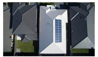
Figure 14: In general, lighter coloured roofs are cooler, with higher SRI
