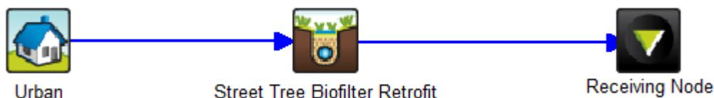
**Figure 3-43 Example of Bioretention Node Application in MUSIC**
