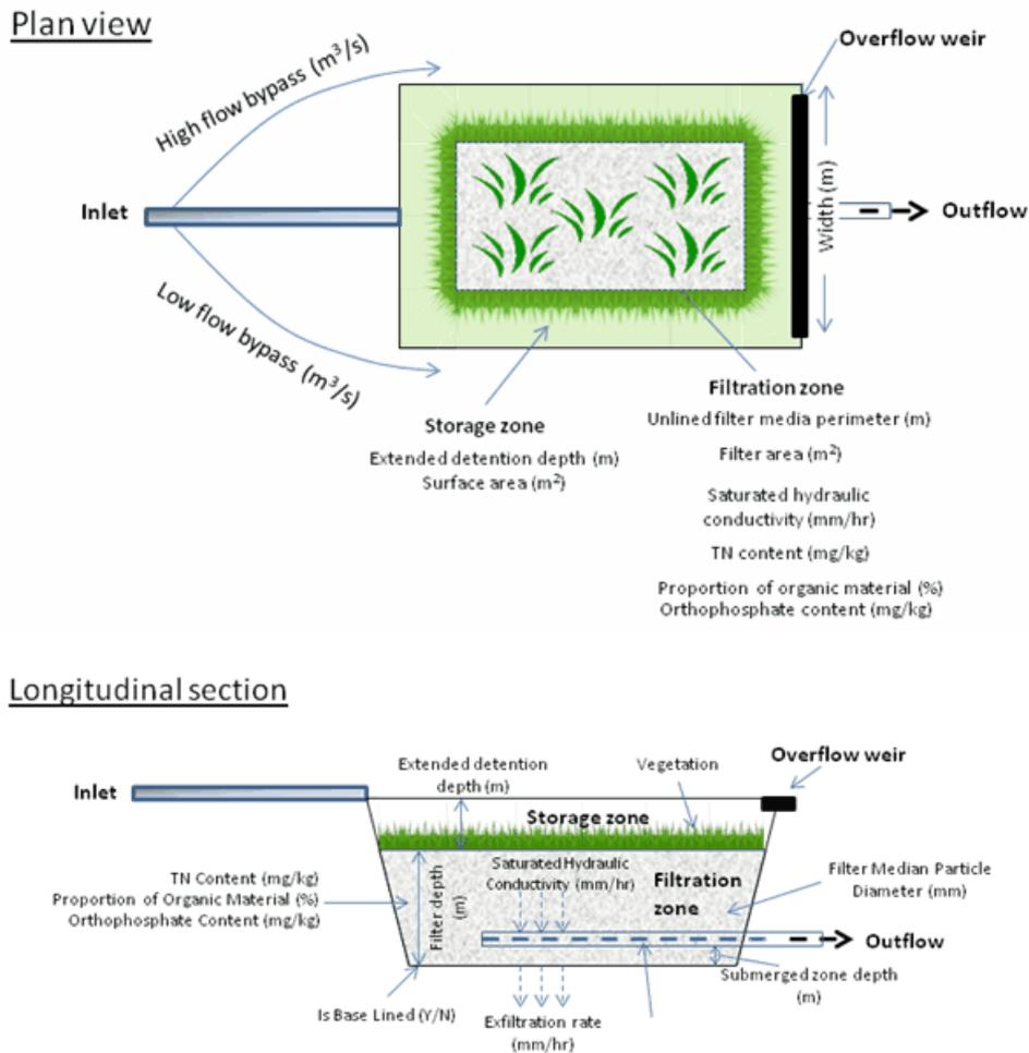
**Figure 3-44 Conceptual View of Bioretention System (as used in MUSIC v4)**
