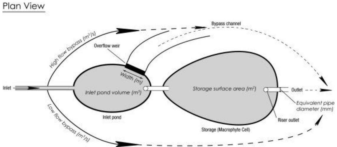
Figure 3-40 Conceptual Plan View of Wetland (as used in MUSIC v4)
