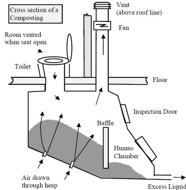
The remaining material slowly moves down a sloping floor by gravity as more material is added to the pile. It then moves under a dividing baffle into the humus chamber as friable compost after about a year.
