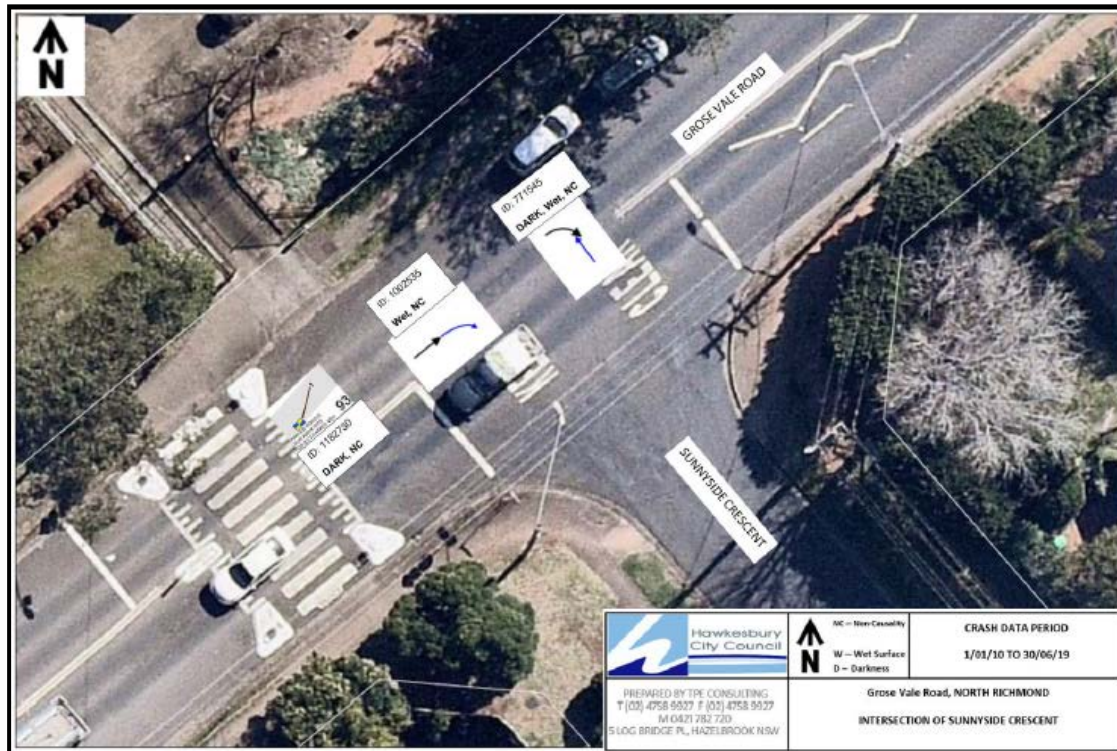
Figure 7: Crash Diagram - Intersection of Grose Vale Road and Sunnyside Crescent, North Richmond
